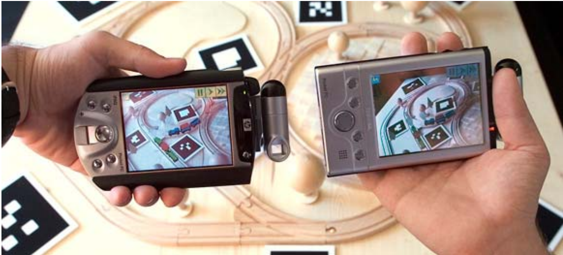
3.8 Gameplay demonstration of The Invisible Train . Individual player's PDAs show live video capture of the real, empty toy train platform overlaid with virtual trains and track switches. (The Handheld Augmented Reality Project, 2004)
